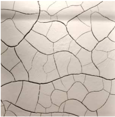
Fig. 1: Typical mud crack pattern in a thin layer of calcium carbonate ( \text{CaCO}_3 ) paste. The thickness was about 4 mm after drying. The width of this photograph corresponds to 10 cm.
